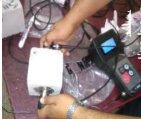
Fig. 3 UPV test at different proportions of concrete with EVA
