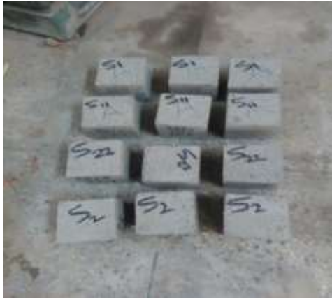
Fig. 2: Sample of concrete mix with industrial EVA
